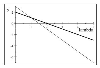
In this graph the thick line is  $\frac{\partial L_{lin}}{\partial x}$  and the thin one is  $\frac{\partial L_{lin}}{\partial y}$ . Notice that while  $\frac{\partial L_{lin}}{\partial y}$  starts out higher by the time it comes to choosing the critical  $\lambda$  (when
